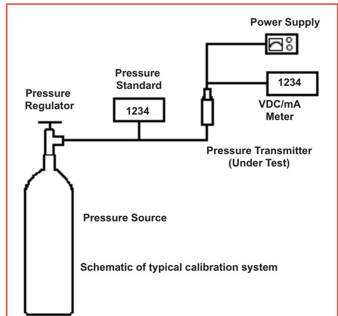
The system should be powered up & allowed to warm up electrically. Typically 10-15 minutes is sufficient. The ambient & process temperature should also be stable. Calibration for standard GP:50 transmitters is done at room temperature, 68 deg F.
