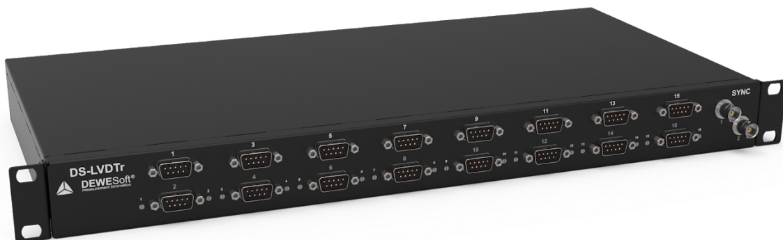
DS-16LVDTTr adapter outputs are located on the front side
