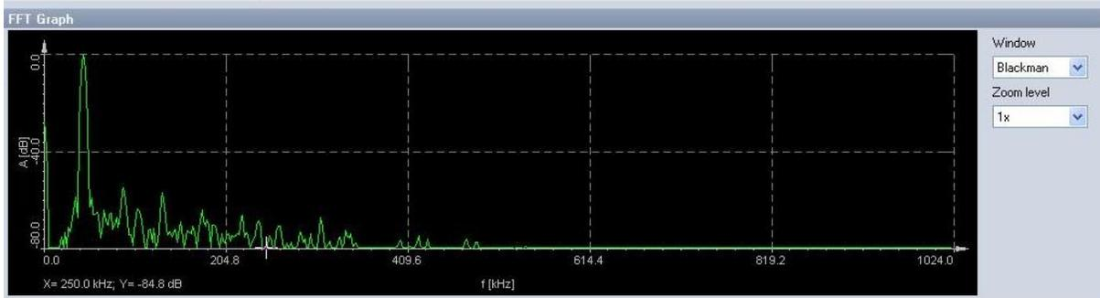
You can hover the mouse over the waveform and the display will calculate the magnitude in dB (vertical Y axis) and frequency (horizontal X axis) and show them numerically at the bottom of the graph.
