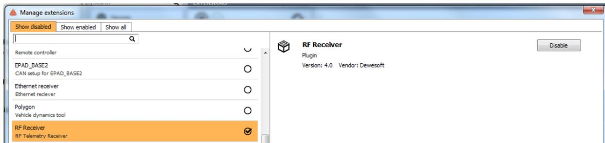
5. In the Extensions pane of the Settings window, locate the Plugins and then RF Receiver. Click on the RF Receiver to examine the settings for the TalonRF. The Plug-In will show how many TalonRF cards are in the system.
