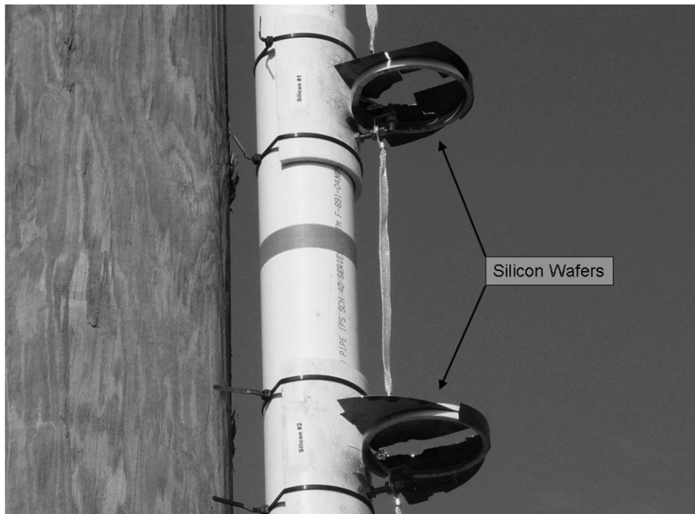
Fig. 6. Lightning-damaged silicon wafers.
