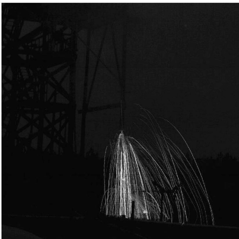
Fig. 8. Integrated video frames showing total luminosity from the silicon particle shower.
