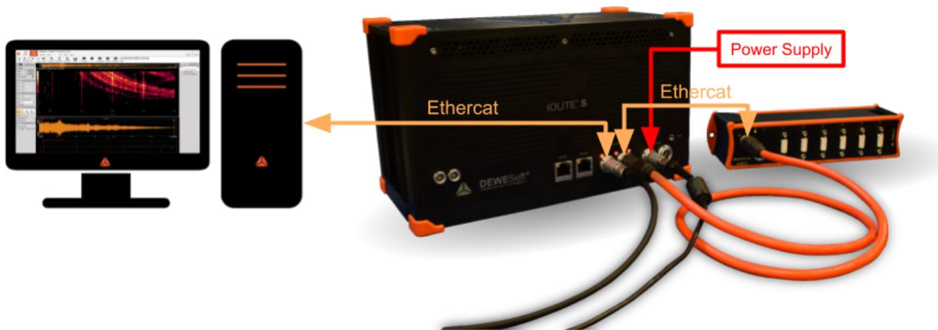
**Illustration 27:** Connection of IOLITEs and KRYPTON<sup>®</sup> device
