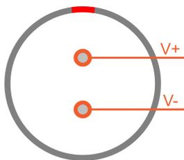
For the power supply an unregulated DC voltage between 12 and 48 Volts is required, which is connected to LEMO 1B connector on the rear side of the chassis.
