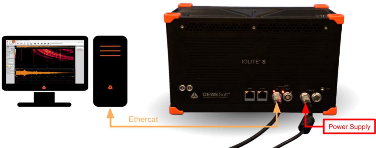
**Illustration 26:** Connection of IOLITEs standalone device to PC
