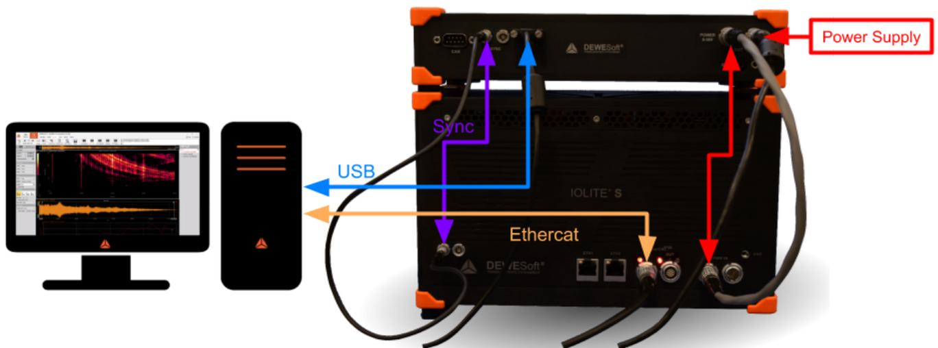
**Illustration 28:** Connection of IOLITEs and SIRIUS<sup>®</sup> device
