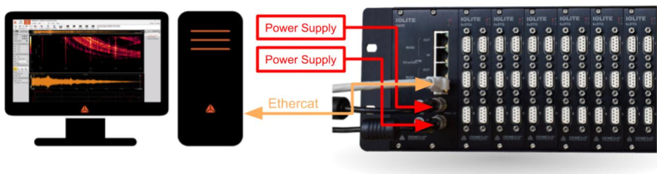
**Illustration 1:** Connection of IOLITEr standalone device to PC
