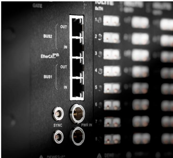
Each IOLITE system has two fully independent Ethercat bus systems that work in parallel.
