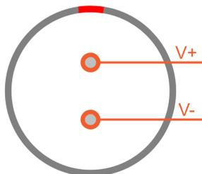
For the power supply an unregulated DC voltage between 12 and 48 Volts is required, which is connected to LEMO 1B connector on the IOLITE-GATE front.
