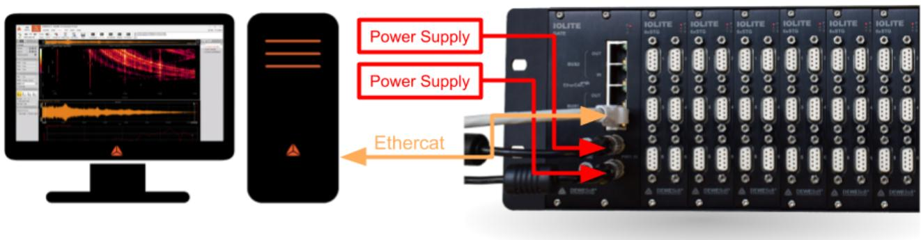
**Illustration 21:** Connection of IOLITEr standalone device to PC
