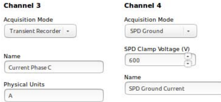
Figure 23: Jupiter TMS channel configuration interface page with SPD Ground Mode selected on Channel 4. Note the additional “SPD Clamp Voltage” numerical input field that was exposed when the SPD Ground Mode selection was activated.
