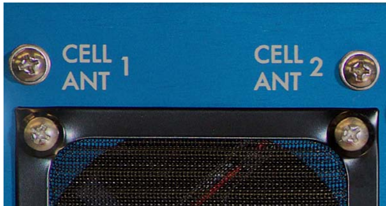
Figure 7: Jupiter TMS cellular antenna connections for an integrated cellular modem. Note that the mounting holes for the SMA female bulkhead feed-through connectors are filled with appropriate fasteners for this Jupiter TMS unit, which did not incorporate a cellular modem.
