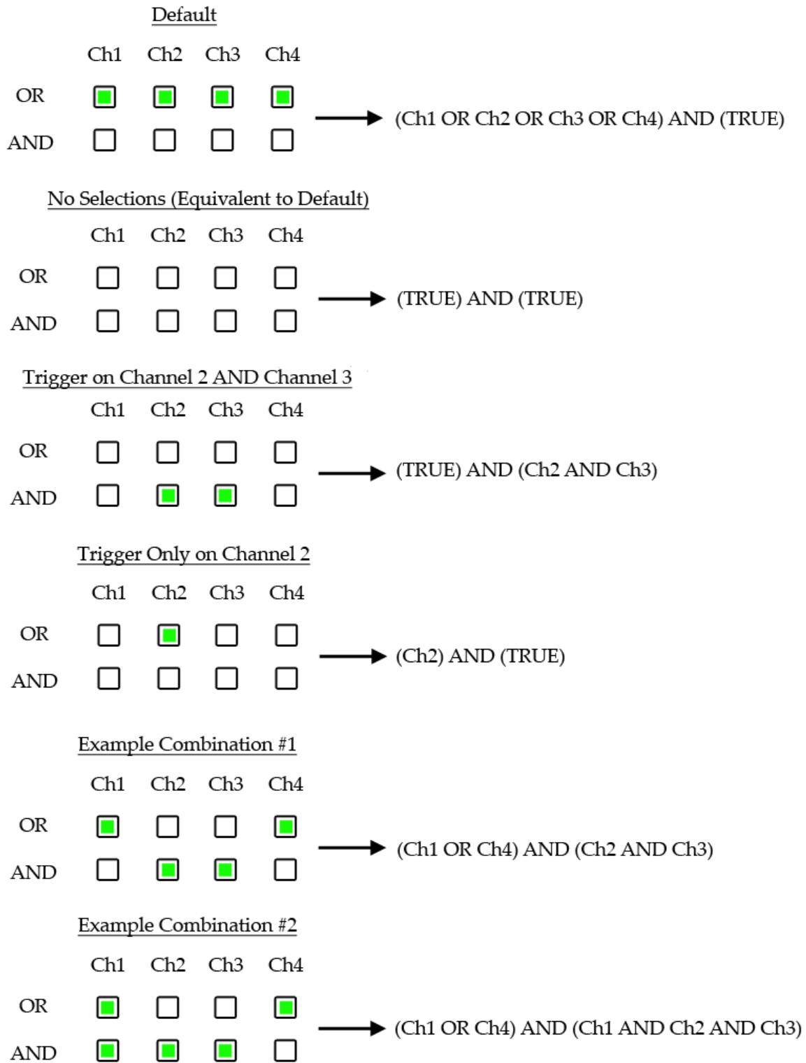
Figure 28: Illustration of Jupiter TMS logic trigger examples for basic and complex trigger schemes.
