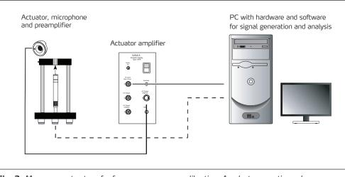
**Fig. 3.** Measurement set-up for frequency response calibration. An electroacoustic analyzer with signal generator can be substituded for the PC.
