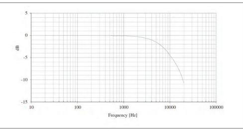
Fig. 4. Frequency response measured with electrostatic actuator.
