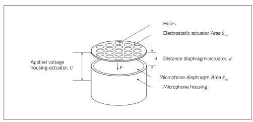
Fig. 2. Principle of microphone excitation with electrostatic actuator.
