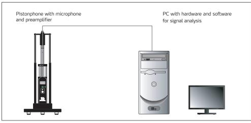
Fig. 1. Set-up for level calibration with pistonphone.
