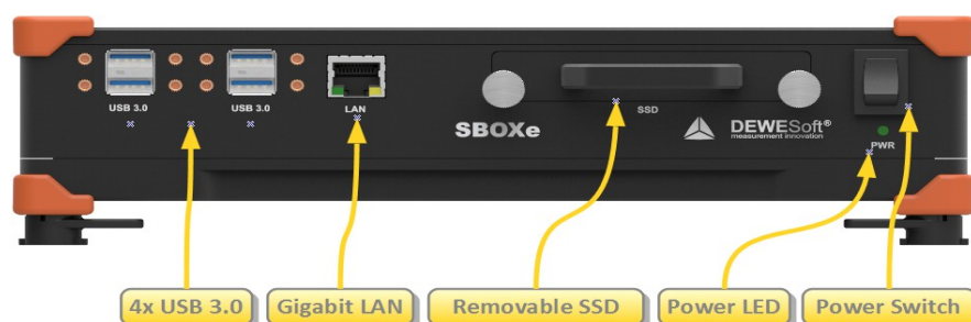
Illustration 62: SIRIUS-SBOXe: Connectors at the front side
