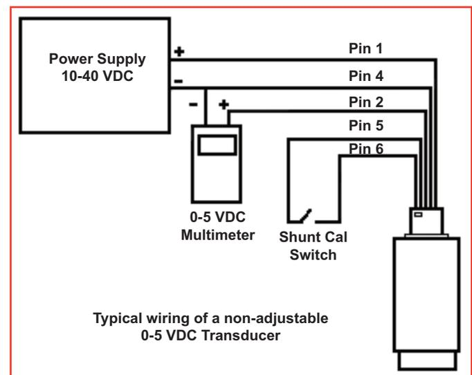
In order to operate these types of devices short or apply power to the appropriate pins. The pin-out can be found either on the performance certificate, marked on the transducers nameplate, our website or by contacting the factory with the model number or serial number.
