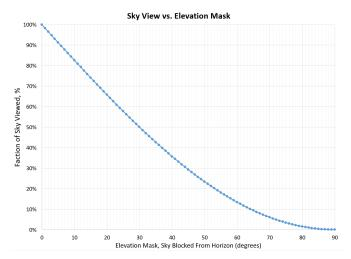
An elevation mask, much like urban canyon environments, eliminates multipath-prone low-elevation satellites, but also limits the amount of sky that can be seen to track remaining satellites.
