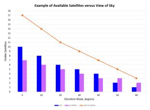
Tracking multiple GNSS constellations provides more satellites in view at higher elevations, as is the case in limited sky-view urban canyon installations.
