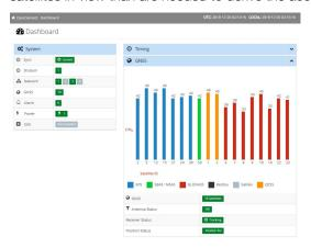
Tracking multiple constellations significantly improves the overall number of visible satellites available to continuously derive the time.
