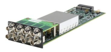
For applications requiring superior low phase noise (LPN) 10 MHz signals, two different LPN modules are available. Each module has eight extremely isolated, phase-coherent 10 MHz LPN outputs, with each module offering excellent levels of LPN or Ultra LPN performance and exhibiting low spurious noise characteristics.
