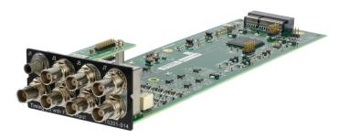
The Standard S650 Timing I/O module is outfitted with an ST fiber connector, replacing the J1 BNC to support input of a DCLS signal over multimode fiber. BNC connectors J2-J8 retain the same functionality as the standard Timing I/O module. The ideal application is slaving an S650 with a Timing I/O Fiber input via the fiber connection to an S650 with a fiber output. The FlexPort license is required with this module as only DCLS signals are supported on the J1 fiber input.
