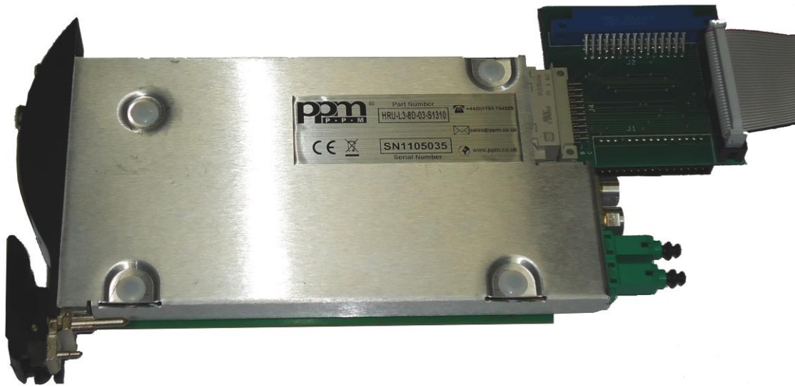
Connection of module interface board to a Plug in module
