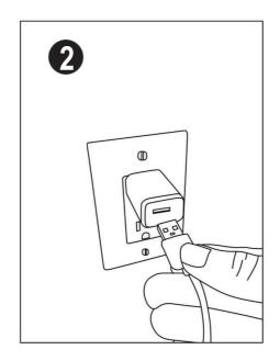
Plug USB cable into USB power supply
