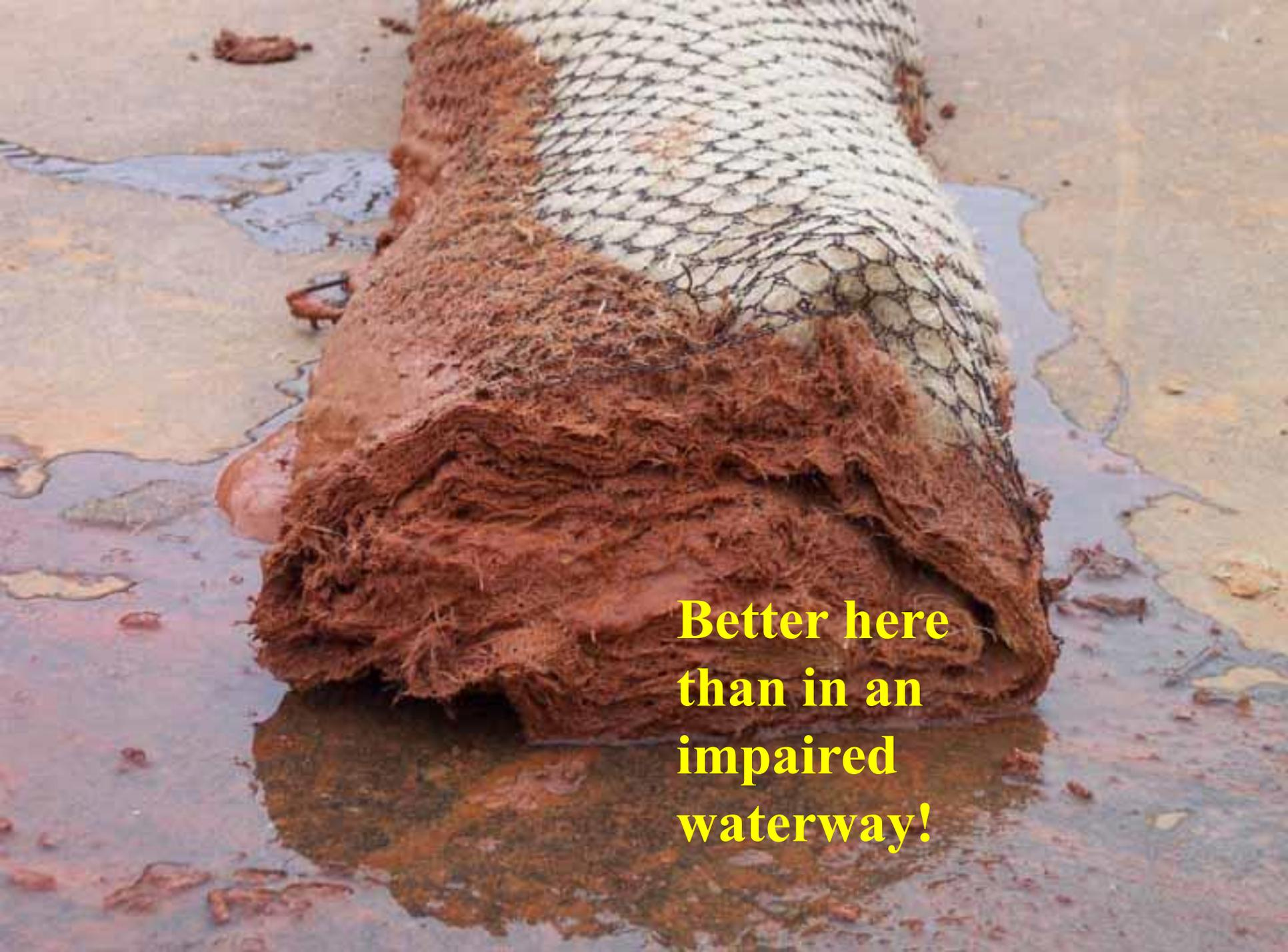
A roll of white geotextile fabric is shown lying on a muddy, brownish surface. The fabric is heavily clogged with thick, brown sediment and debris, particularly at the bottom edge. The surrounding area is wet and muddy, with some puddles of water reflecting the light. The text "Better here than in an impaired waterway!" is overlaid in yellow on the bottom right of the image.
