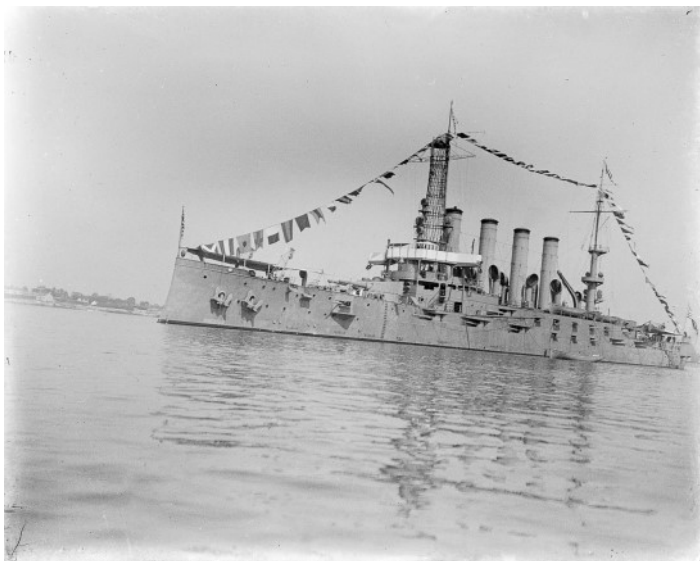
California Class built between 1903 and 1905. Length 502 ft beam 69.5 ft.. Classified as an armored cruiser, there were 6 ships in this class.
