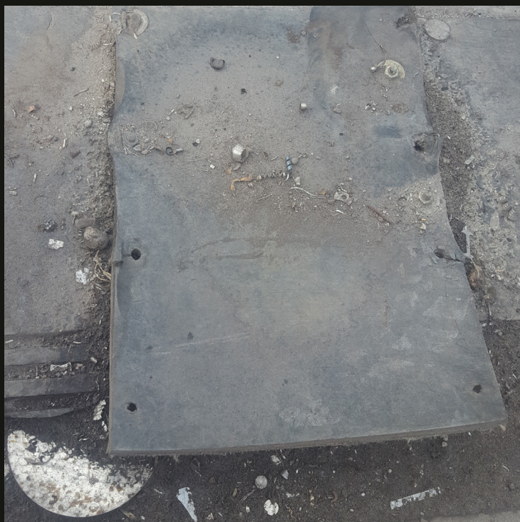
Before: Damaged panzer belt due to abrasion
