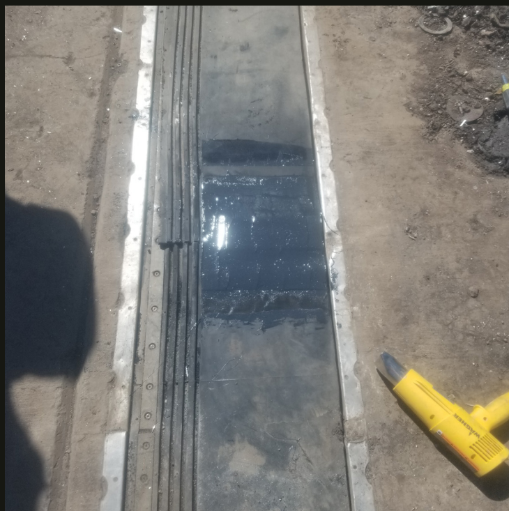
After: Panzer belt repaired with Belzona 2211 & Belzona 2911
