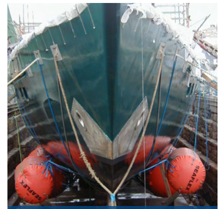
Anchor pocket bonding completed
