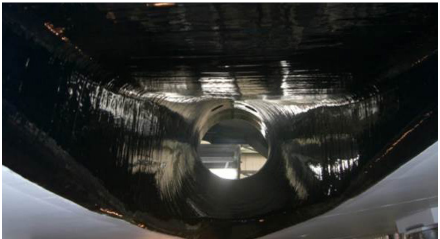
Cavitation protection coating applied to jet tube area on super yacht
