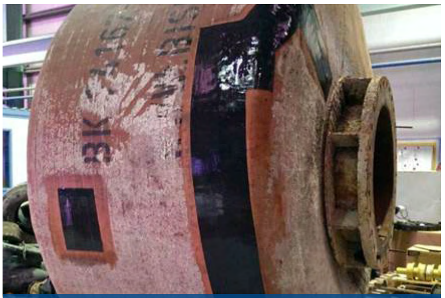
Damaged areas repaired
