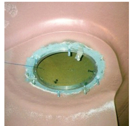
Rudder bearing bonding - bottom view
