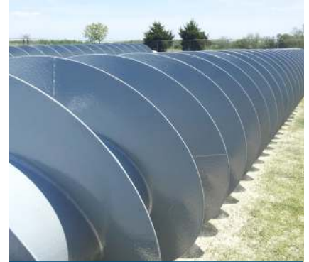
Erosion resistant coating applied
