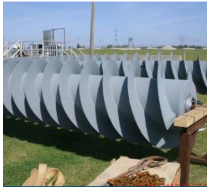
Screw conveyors prior to coating
