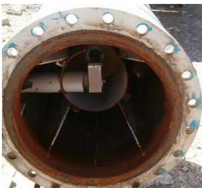
Corrosion and erosion on internal surfaces caused by sewage water
