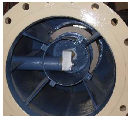
Internal surfaces rebuilt and protected with Belzona coating
