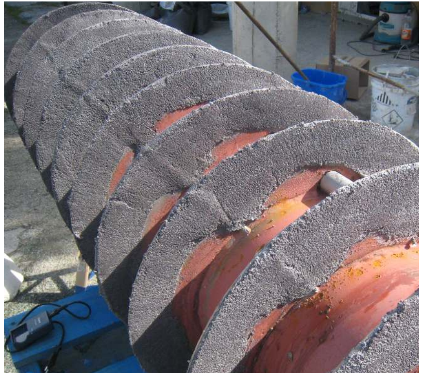
Belzona abrasion resistant coating extends the life of screw conveyor
