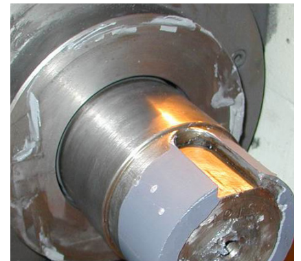
Keyway housing and shaft repaired with Belzona material
