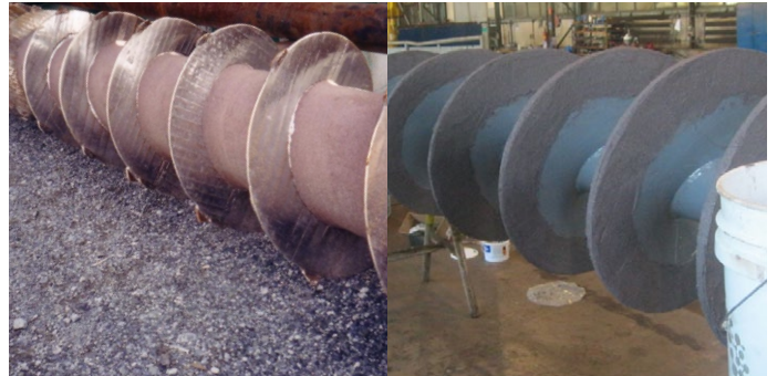
Archimedes screw protected against abrasion
