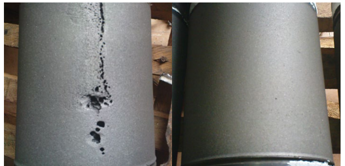
Wet cylinder liner refurbished
