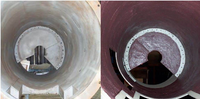
Mixer rebuilt and protected against abrasion
