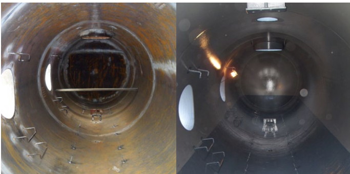
Vessel lined for corrosion protection at elevated temperatures
