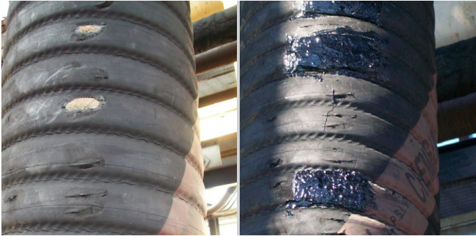
Oil suction and discharge hose repaired
