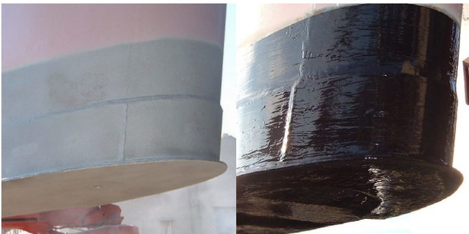
Ships rudder protected against cavitation
