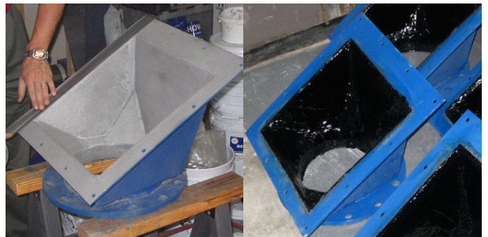
Hoppers lined for abrasion protection
