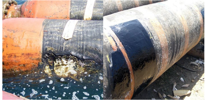
Damaged floating hose restored
