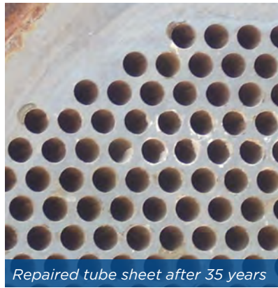
HEX head repaired and protected
