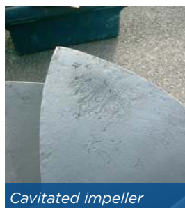
Erosion on internal surfaces of pump
