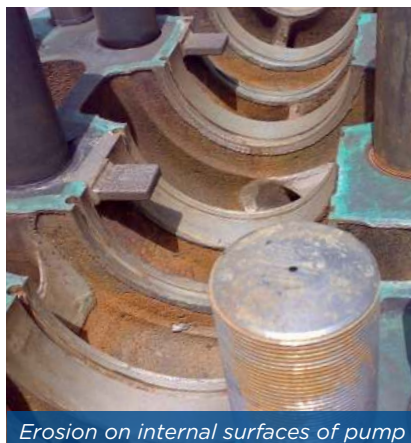
Erosion on internal surfaces of pump
