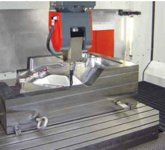
Machining of large dies and extra-dimensioned components are carried out efficiently by the KR configurations.
