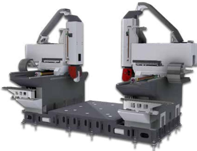
FIDIA's experience as the sole supplier of an overall solution has made possible this particular configuration: two standard systems, with a shared cast iron table, doubling productivity with respect to other gantry systems having a similar work volume.
