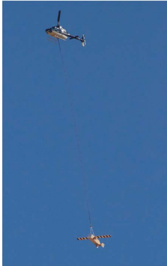
Figure 6. 100% scaled glider attached to 100 ft sling.
