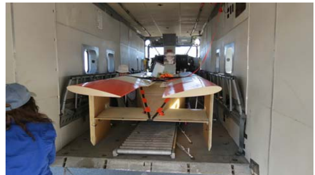
Figure 9. Glider installed inside SC-7 Skyvan.
