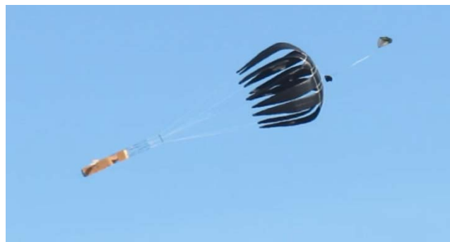
Figure 5. Parachute Landing uses a GFE Low Cost High Velocity (LCHV) Chute.
