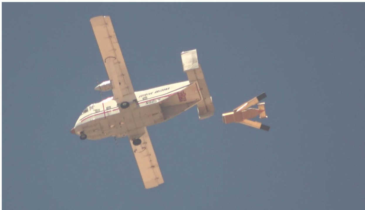
Figure 1. LG-2K RAIN glider released from a Shorts SC-7 Skyvan cargo aircraft.
