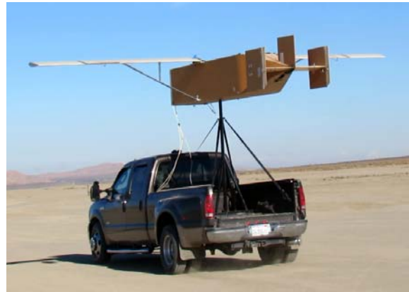
Figure 7. 100% scale prototype glider on top of a 7-ft high truck mounted test stand.
