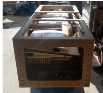
Photo of LG-1K TACAD glider with top loading hatches and nose removed to show component storage
