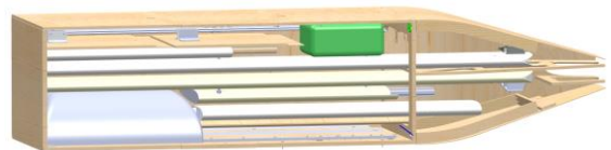
LG-1K TACAD fuselage as a shipping container is 9 ft (2.74 m) long
