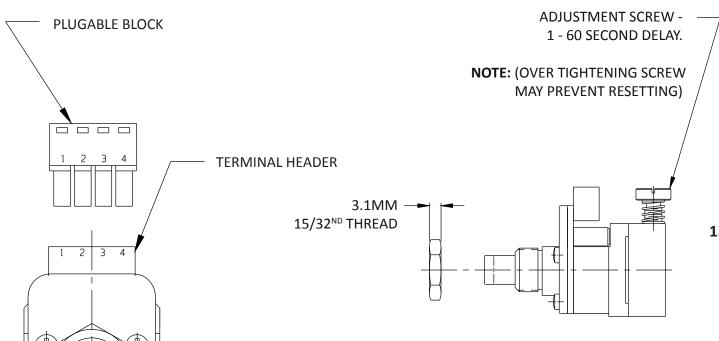
1. TERMINAL PINS 2 & 3 NORMALLY OPEN PINS 1 & 4 NORMALLY CLOSED.
