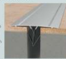
W-90 installed over 25mm joint width using small clip option.
