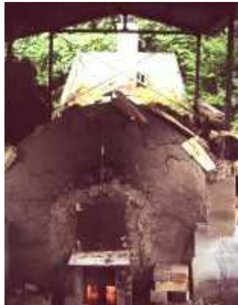
A hobby kiln (Shigaraki-style anagama) of a Tokyo school teacher friend of the Shigetoshis in the third day of an eight day firing. The kiln is in the next prefecture, a short distance from Mashiko.
