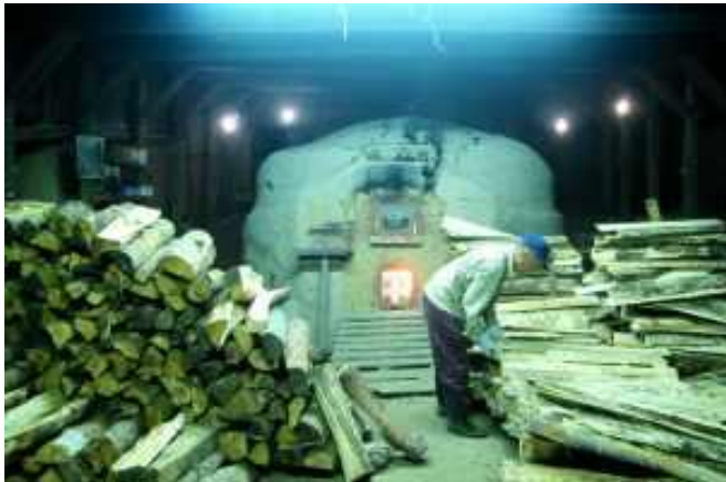
One of Ryoji's three noborigama kilns at Kanayama fired for five to six days with red pine found near Goshogawara.
