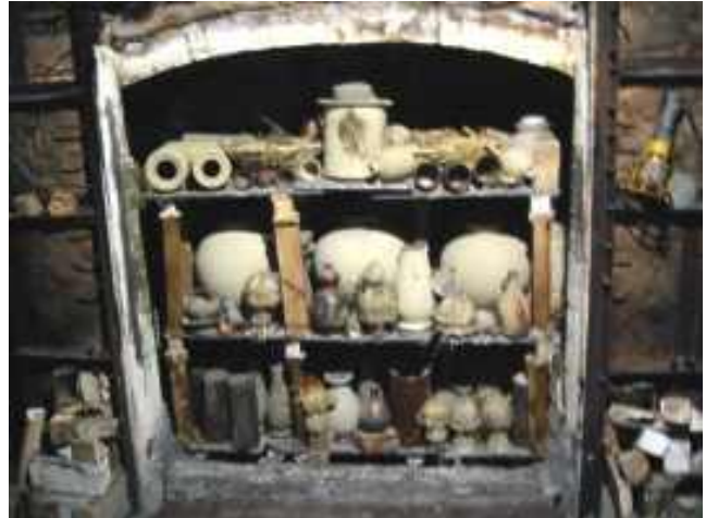
This is a view into a smaller gas kiln where Setsuo achieves Bizen yaki effects by using rice straw and charcoal introduced at the end of the firing. Setsuo has a large anagama kiln, perhaps about 10 metres in length, also at his Kurashiki studio.
