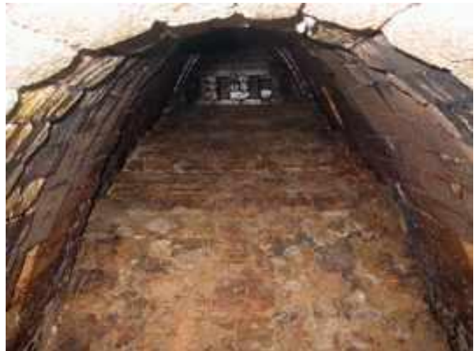
The interior of Owen's anagama. He fires it for about 100 hours to achieve spectacular and subtle woodfired effects.
