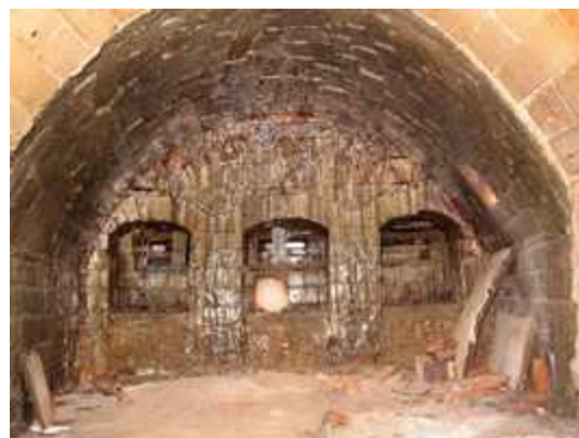
The interior of the large firebox of Robert's kiln, where he sometimes pulls over large vessels at the end of the firing to submerge them in charcoal and ash.
