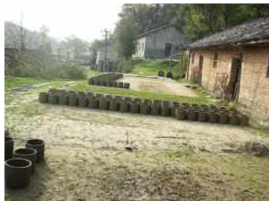
Roof tiles, first made in a bucket mold and then quartered for drying and firing.
