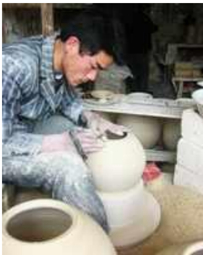
Trimming the leveled join area for the addition of the top.
