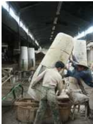
The split half molds have pipe handles for the four workers to move them to the drying area.
