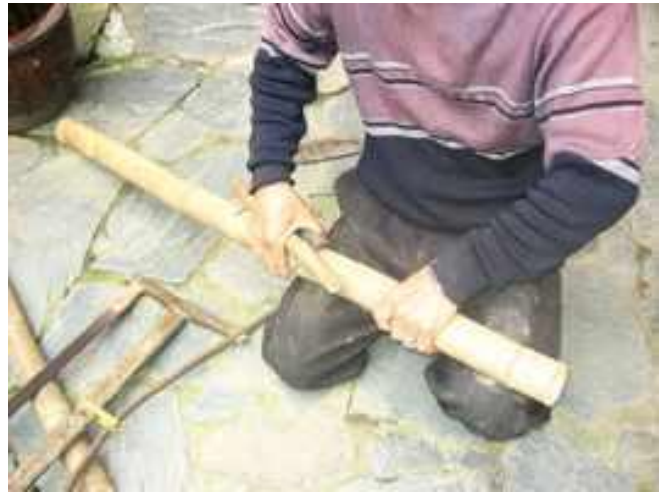
He used a draw knife plane to smooth the joins in the bamboo.
