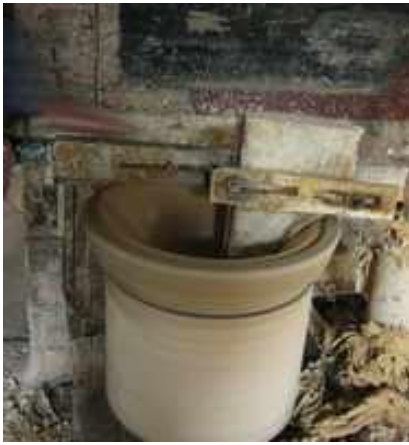
The tops of the vases are jiggered.
