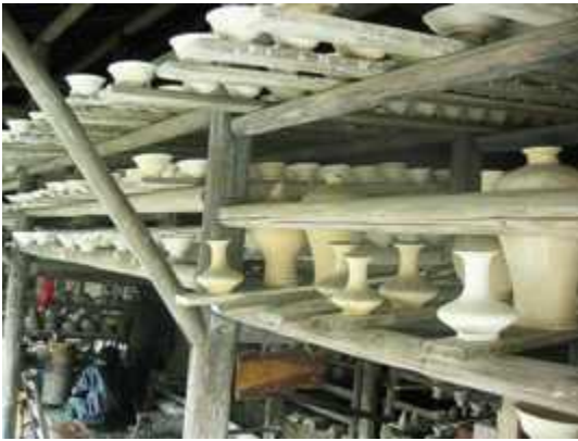
Thrown and trimmed ware awaits glazing on drying racks.
