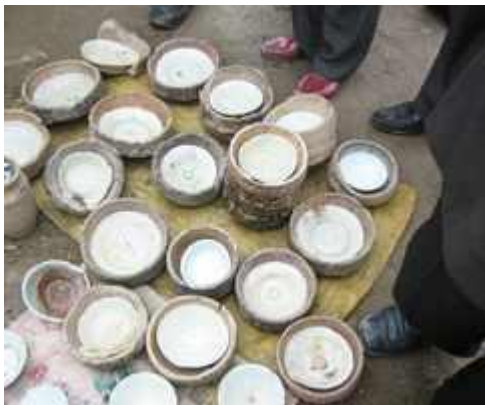
Sometimes the saggars would be fused together - almost always the bowl inside was fused to the sagger. The saggars were often cut apart with a diamond saw.
