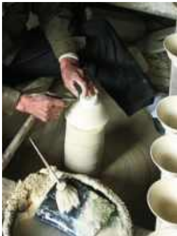
After a brush of water the dry bowl is trimmed and footed.
