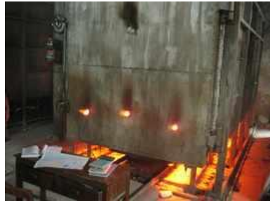
One of the many trolley shuttle gas kilns firing in Jingdezhen. We fired our work in these kilns, sometimes to 1300C and sometimes to 1330C. They crash cool these kilns for brilliant colors, usually depending on how many large deity sculptures are in the load. The turnaround time is one day - loading to unloading.
