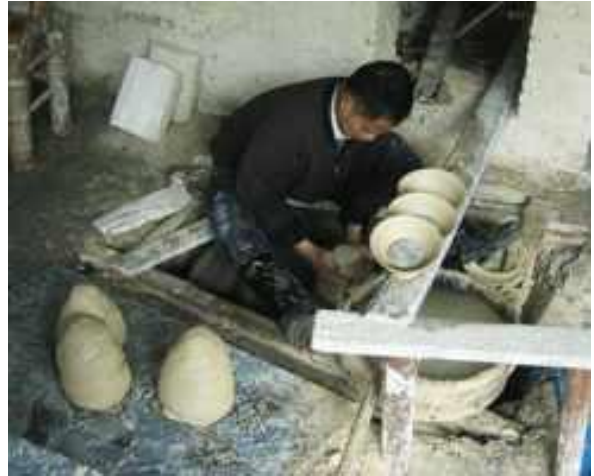
Bowls thrown off the hump of porcelain on a stick powered wheel.
