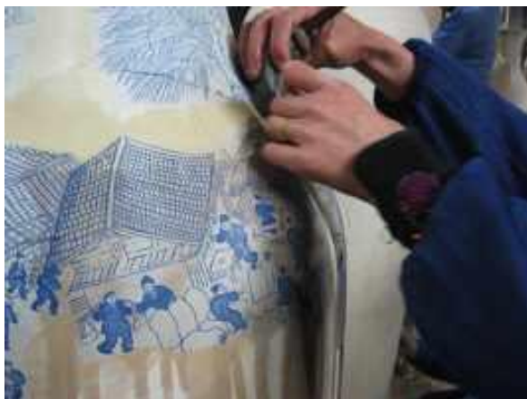
Underglaze decals were used on most, applied freely in a collage style to a pre moistened spot and then the wet paper removed.
