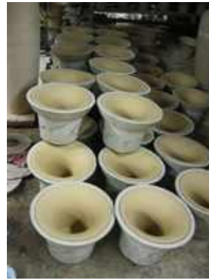
These jiggered pieces are then paired up to form the vase top addition.
