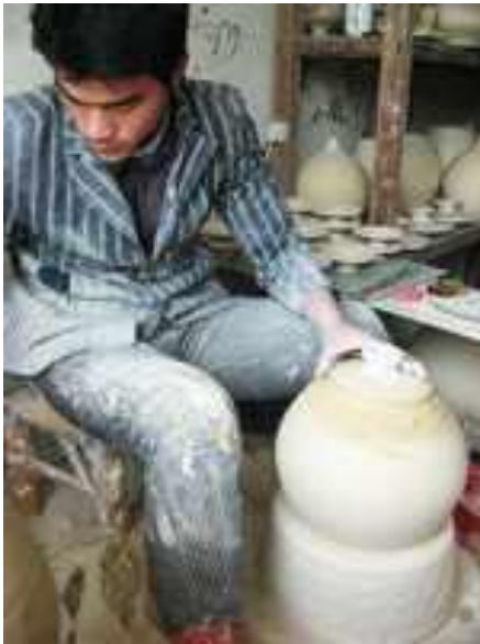
Thrown bottle top section centered on body in trimming chuck.
