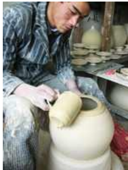
Slip added to dry body to adhere top section.
