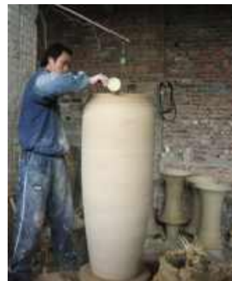
A cup of slip is applied to the top of the dry body. The two part joined jiggered vase tops are in the background.
