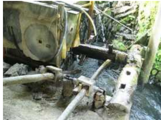
The spokes on the timber axel depress and release the pounder shafts as the axel rotates.
