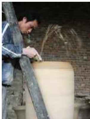
Once removed from the mold the body is turned on a trimming wheel where it is brushed with water and a level joining surface is turned.
