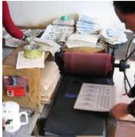
Decal sheet is ready for the press
