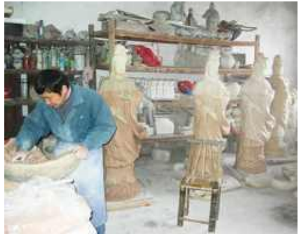
Press molding a portion of Kuan Yin's body in plaster mold.
