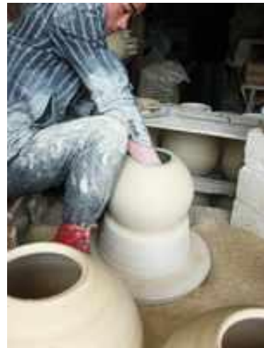
Trimming the dry vase, both inside and out, in a trimming chuck.
