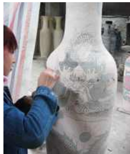
Sometimes the deco was from a pounced template and then hand painted and at other times a carved deco was used.
