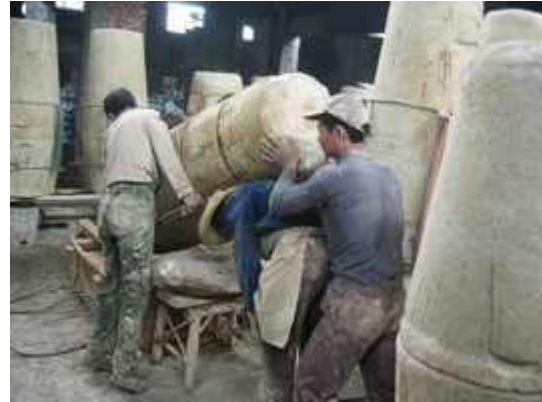
Back breaking work to empty the large mold.
