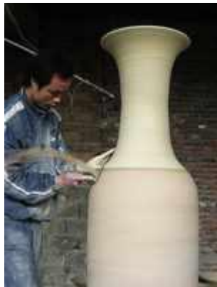
After placing the top on the base, the unit is trimmed to form a continuous curved join.
