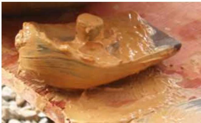
"Cow's tongue" wooden rib used for forming tea bowls.
