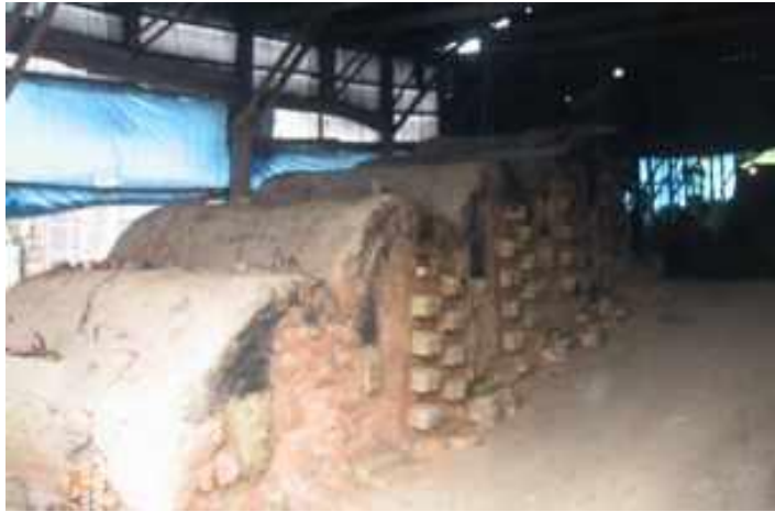
The climbing kiln with the charcoal stoke hole bricks in place.
