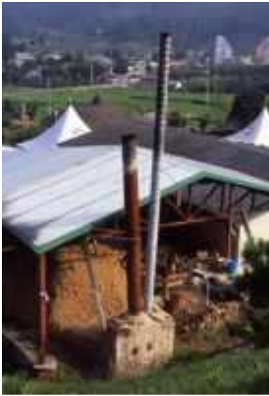
The double chimney of Moon's kiln in Joryung.
