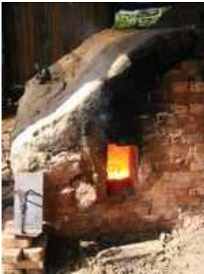
The stoke hole in the firebox of the climbing kiln.
