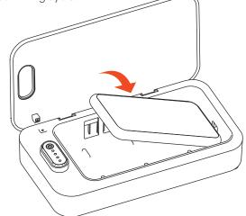
**Note:** The UV-Zone will not work if the lid is not completely closed during use.
