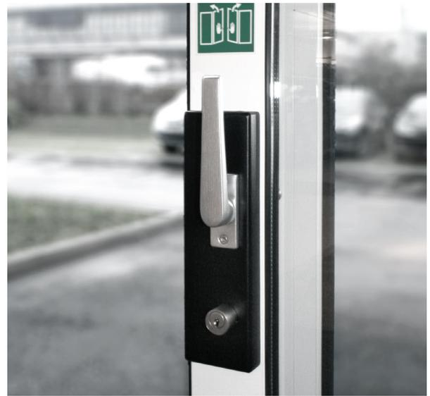
**The Gilgen multipoint locking FLUVERI is a high quality lock system that guarantees fast and safe locking and unlocking of the door. It is invisibly incorporated into the vertical profile of the door leaves. Thanks to the pivoting locking bolts, the door is efficiently protected against forced opening attempts using lever action from any direction. As an option, this system can be complemented by a door and lock-monitoring feature.**
