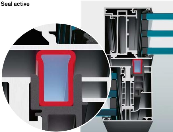
By pressing the button, air is introduced into the frame and the seal is pumped up. The seal presses against the sliding profile and closes the gap between the slider and the fixed frame to create a perfect seal.
