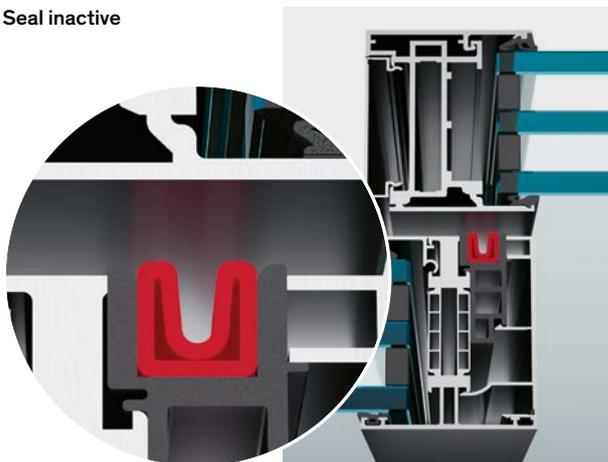
The button is pressed a second time to open the unit. The air leaves the unit and the seal retracts to its original concave profile.
