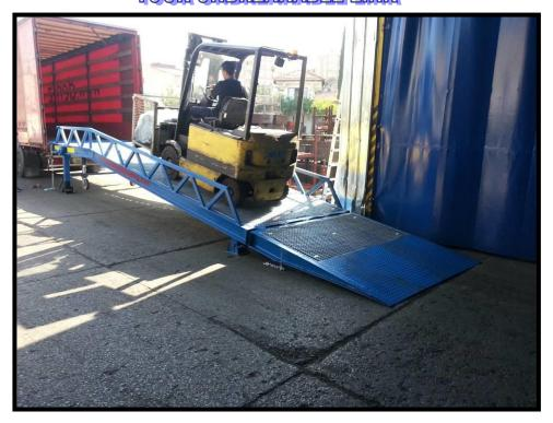
**Safety and Security;** Side barrel and safety chain that is used quick lock for fixing the mobile yard ramp to the container/truck serve extra ordinary safety properties to customers. Reinforcement hinged lip supply extra safety when forklift is operated. We have manuel front **support legs** for enhancement safety at middle axle model. **On the contrary** of our competitors we only used galvanised rainforced metal gril this special system blocked slippery ever conditions .
