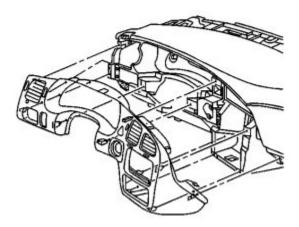
10. After removing the trim plate bezel simply remove the four ¼" screws holding the instrument cluster in place. Pull the cluster out and unplug the single wiring harness connection in the back.
