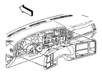
6. After removing the trim plate bezel simply remove the four ¼" screws holding the instrument cluster in place. Pull the cluster out and unplug the single wiring harness connection in the back.
