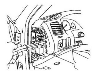
6. Remove the screw from the left side of the IP cluster trim plate.
