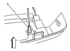
11. Disconnect the I/P compartment light electrical connector (1).
