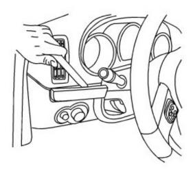
4. Remove right trim panel, first removing HVAC knobs
