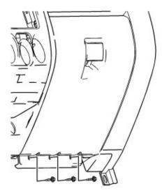
6. Remove left side knee bolster. Remove 3 screws holding knee bolster to instrument panel
