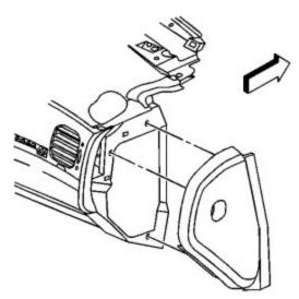
6. Remove the instrument panel (I/P) fuse block access hole covers.
