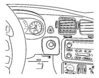
2. Using a small flat-bladed tool, remove the bezel from the ignition switch cylinder.
