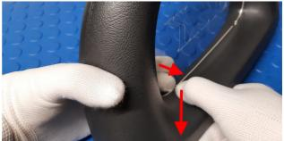
The retaining lugs are rounded and will not damage your roll bar. They hold the insert in the foamed casing in a form-fitting and non-positive manner. After dismantling, the small pressure points disappear completely within a short time.
