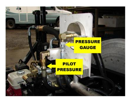
Using 2 wrenches (one to hold the part, the other the fitting) loosen the fitting on the back of the pressure gauge WHILE pressurized fluid is supplied to the system. Wrap a rag around the fitting and CRACK the fitting JUST A WEE BIT! Any air bubbles in the line will burp out and clean fluid will flow from the fitting. Tighten the fitting while fluid is flowing.
