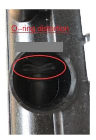
**Solution:** Replace with new O-ring. When installing, properly brush a little coolant to the O-ring for better greasing.
