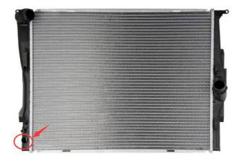
**CAUSE**: the drain plug was improperly installed, which distorted the O-ring resulting in loss of sealing effect.
