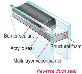
The result is an unbelievably durable double seal that provides for amazingly consistent seal quality.
