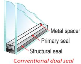
Super Spacer, however, reverses the process. Its structural seal is on the inside – pre-applied to the spacer itself. This takes the form of a pressure sensitive, acrylic adhesive backed up by hot-melt butyl or a comparable, low permeable sealant on the outside, where a gas/moisture barrier seal can do the most good.
