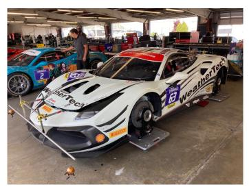
To start, you need some method of setting the strings along either side of the car. The strings have to be exactly parallel and should run approximately through the center of the front and rear hub as far as vertical orientation.
