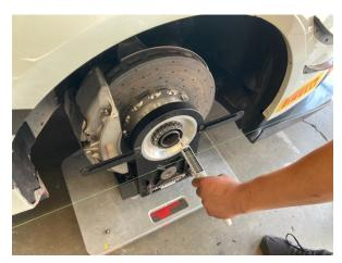
To center the car on the strings, you should take a measurement with your StringStick<sup>tm</sup> from the wheel hub to the string on each side and then very carefully move each bar from side to side until the distance from the hub to the string is identical on both sides. You will need to do this for both the front and the rear hubs.
