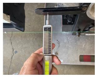
The number that you see on the scale only relates to other numbers nearby, so you can use any portion of the scale. If, for example, the rear reading was 55.5 millimeters and the front reading was 54.5 millimeters then you would have 1 millimeter of toe out on that side of the car.
