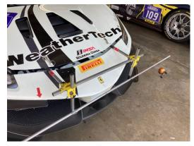
As far as the strings themselves, I like fluorescent mason's string, as the edge is free from fuzz and highly visible. However, many prefer fluorescent monofilament fishing line and tend to center the line on the marks on the scale, as opposed to using the side of the mason's string. With either, a fishing reel is a good way to store the string.
