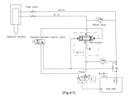
Fig.4-1 is shown the one of simplest hydraulic circuit in case of installation a service port into the main control valve of base machine.
