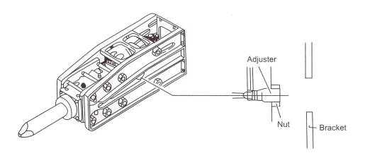
The cylinder adjuster is installed to the right side of the cylinder.
