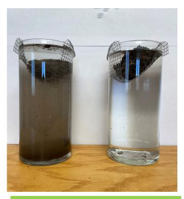
Slake Test- this is an easy test you can do to show the stability of your soil clods. The soil on the right has been no -tilled since the early 1980s and the one on the left is in a seed corn and soybean rotation with multiple tillage passes every year. Once dropped in water, the forces of the water moving into pores breaks apart the weak structure of the soil on the left.
