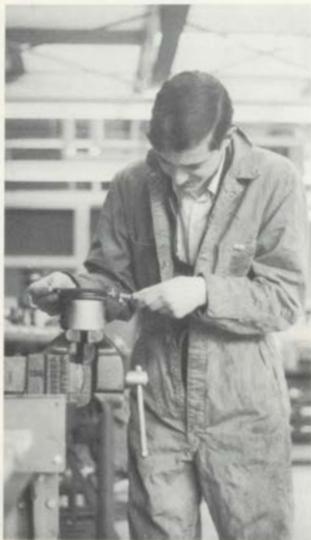
Precision is an important part of auto shop work, as Mike Hanselman knows. Thus, he makes doubly sure to get a piston ring fitting properly.
