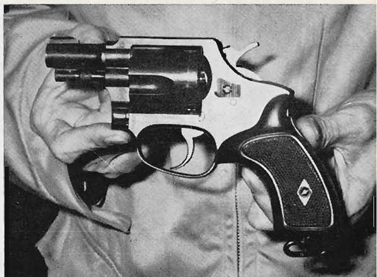
This new Nambu Model 60 is chambered for the .38 Spl., holds five rounds, and looks very much like famed U.S. snub-nosed revolver. Gun has automatic hammer safety, but otherwise is built along the conventional lines.
