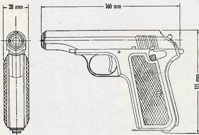
This new Nambu Model 57 B is the 7.65 mm pocket auto pistol. The clear plastic grips permit seeing function of the magazine disconnect safety. Gun points well, handled nicely on range, placed shots satisfactorily.
