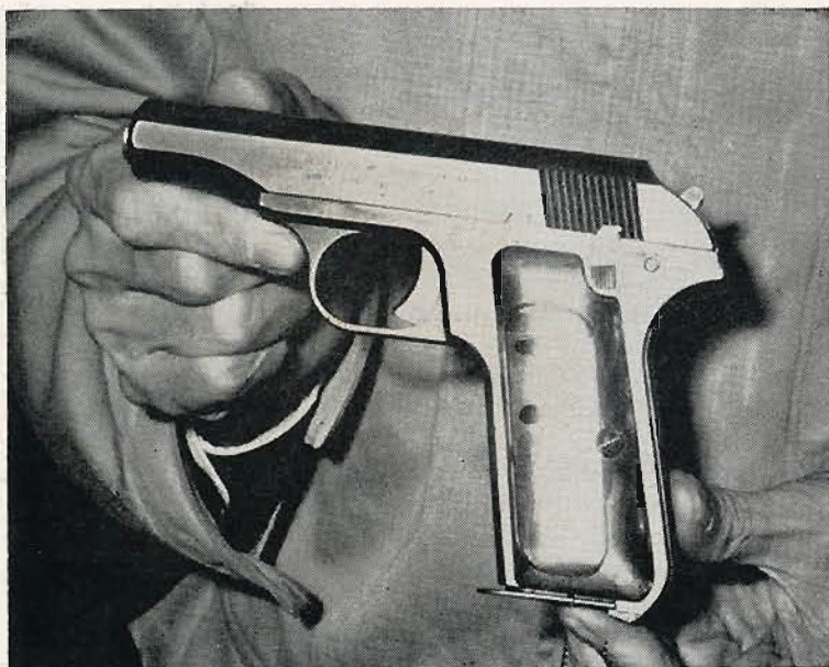
This new Nambu Model 57 B is the 7.65 mm pocket auto pistol. The clear plastic grips permit seeing function of the magazine disconnect safety. Gun points well, handled nicely on range, placed shots satisfactorily.
