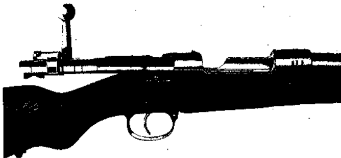
MODEL 98. GERMAN INFANTRY RIFLE. RIGHT SIDE VIEW OF RECEIVER WITH ACTION OPEN READY FOR LOADING
