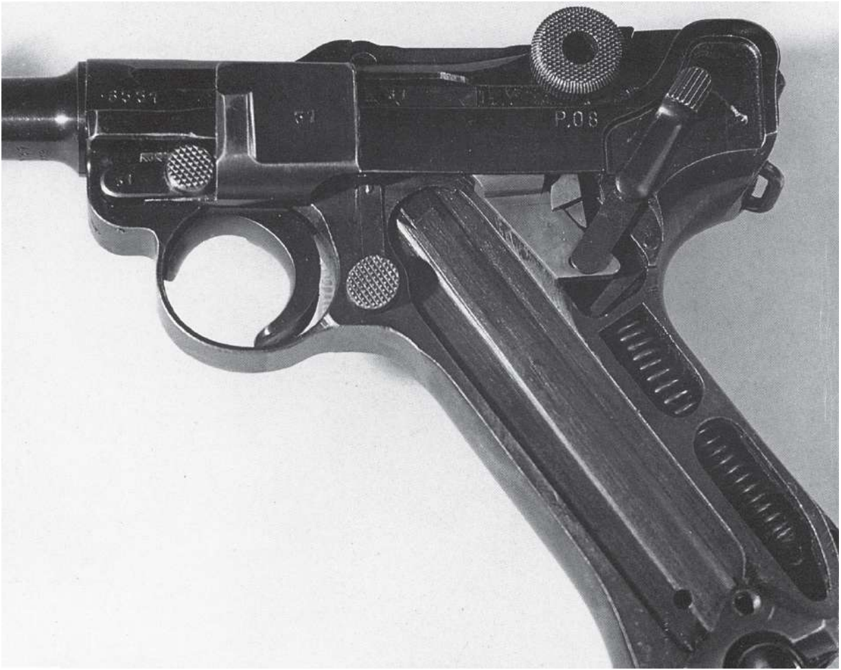
Plate 76 The Martz Safe Toggle Release installed in a wartime German P.08. Note the alteration to the safety-lever mechanism behind the magazine. John V. Martz.
