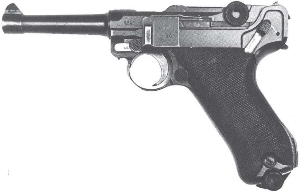
Plate 58 This Luger – no. 4640f – was made by DWM in 1918, but has the additional ‘1920’ property mark above the chamber. It also has a Schiwy sear safety above the trigger plate, showing police usage.
