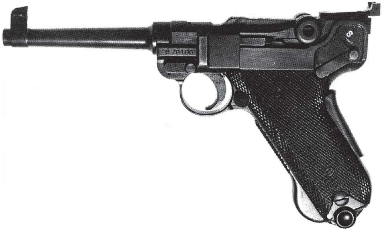
Plate 68 This experimental target-shooting version of the Swiss 06/29 Luger, P78106, was made in the Bern small-arms factory in 1947. Note the sights and the extension on the front grip strap.
