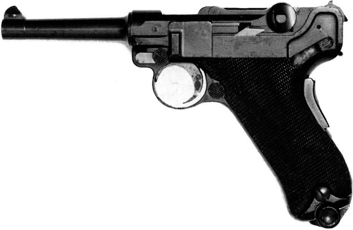
Plate 4 Amongst the earliest Lugers to be tested by the German army was this 9mm Old Model, no.22539, which dates from 1904. An inspector's mark is visible ahead of the trigger plate. Dr Rolf Gminder.
