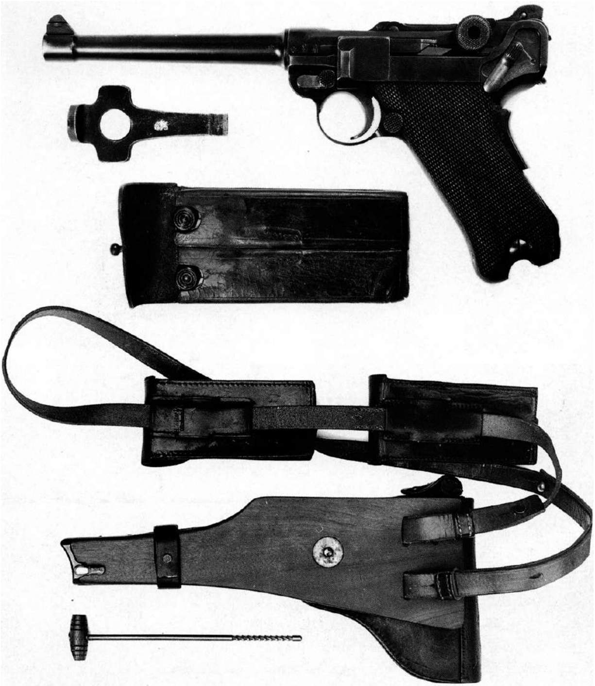
Plate 11 Pistolet 1904 no.3173a, an original 1906-type gun with an altered safety catch, is shown here with a holster, a board-type shoulder stock, a shoulder strap, and spare magazine pouches. One pouch clearly displays the
