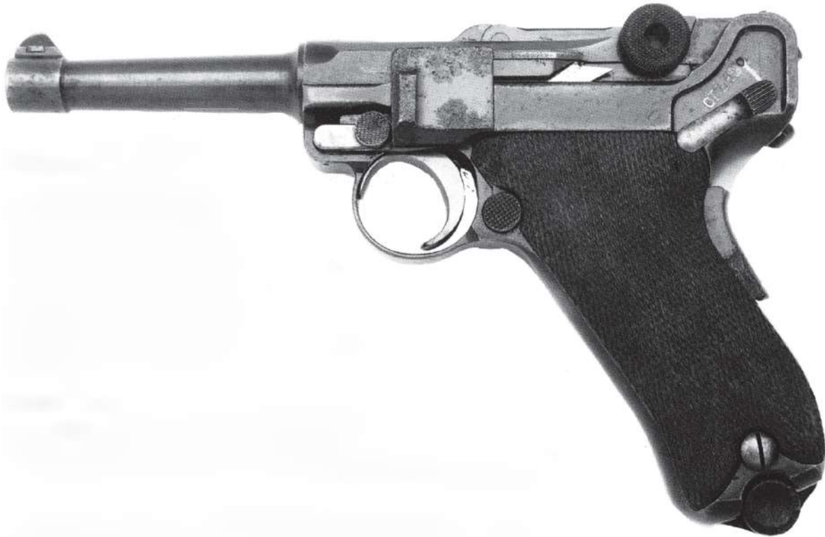
Plate 16 Showing evidence of hard use, this Bulgarian Luger, now no. 1267, was originally a 7.65mm 12cm-barrelled gun supplied about 1907. It has been converted by substituting a 9mm-calibre 10cm barrel, apparently in the early 1940s. Dr Rolf Gminder.
