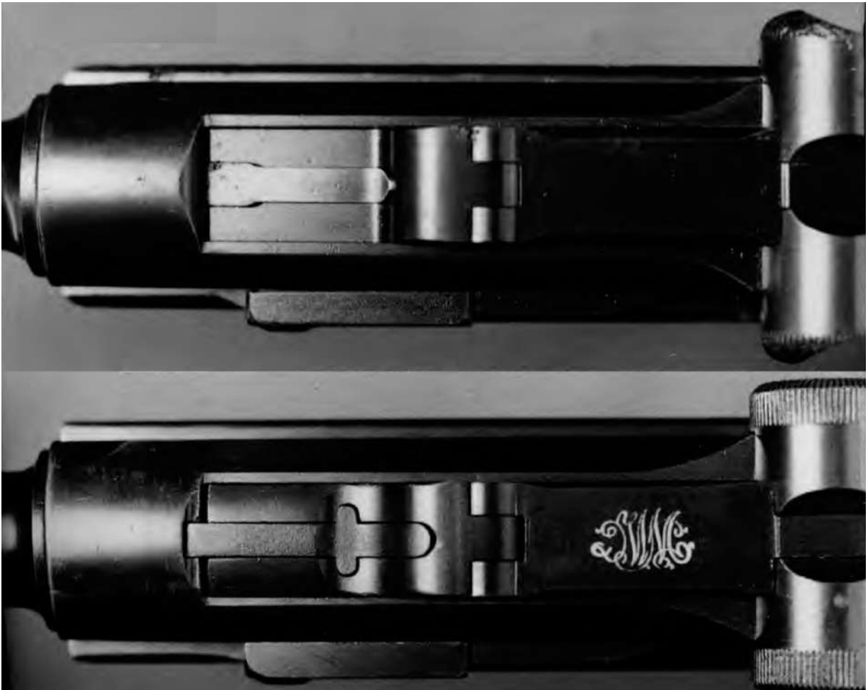
Plates 12,13 The advent in 1904 of the combination extractor/loaded-chamber indicator was accompanied by a major redesign of the breechblock. The photographs show the difference between the Old Model flat variety (12) and the sculpted New Model (13). Dr Rolf Gminder.
