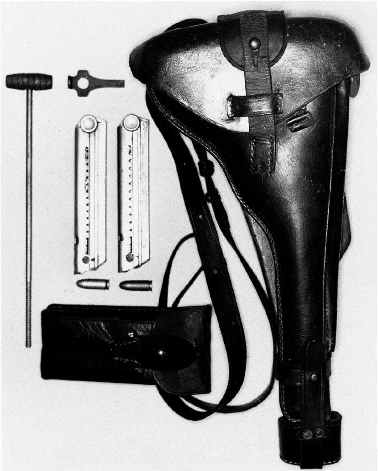
Plate 32 The holster and shoulder-stock unit of the LP.08, with accessories. The holster was made by Mühlendorf & Co. of Barmen in 1918. Per
