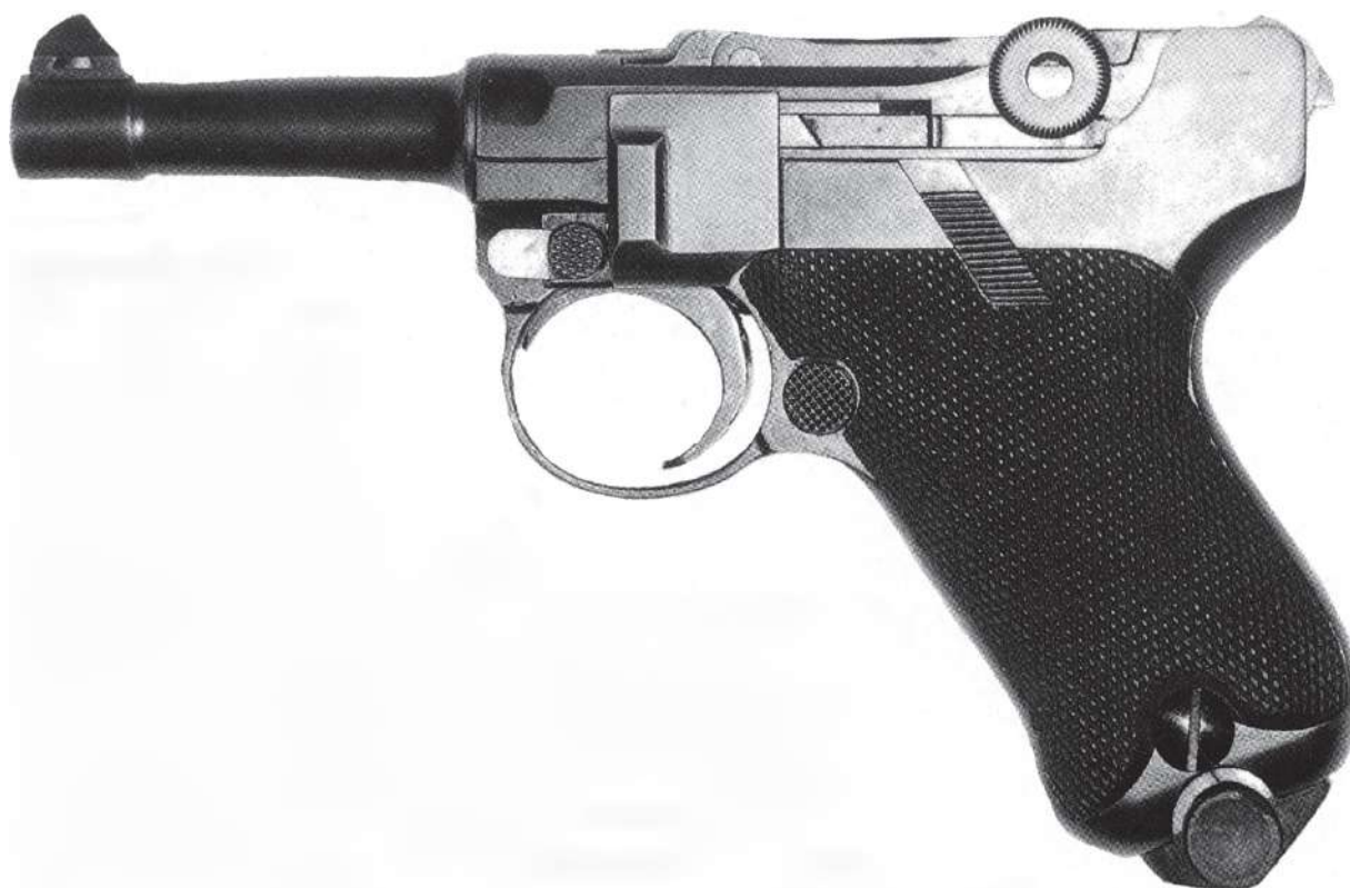
Plate 42 Only four 'baby Lugers', two each in 7,65mm Auto and 9mm Short, were made in the mid 1920s. The flat-surface frame and the sliding Borchardt-type safety catch are most distinctive. This is the only known survivor. Carl Wilson, via Joseph J. Schroeder.
