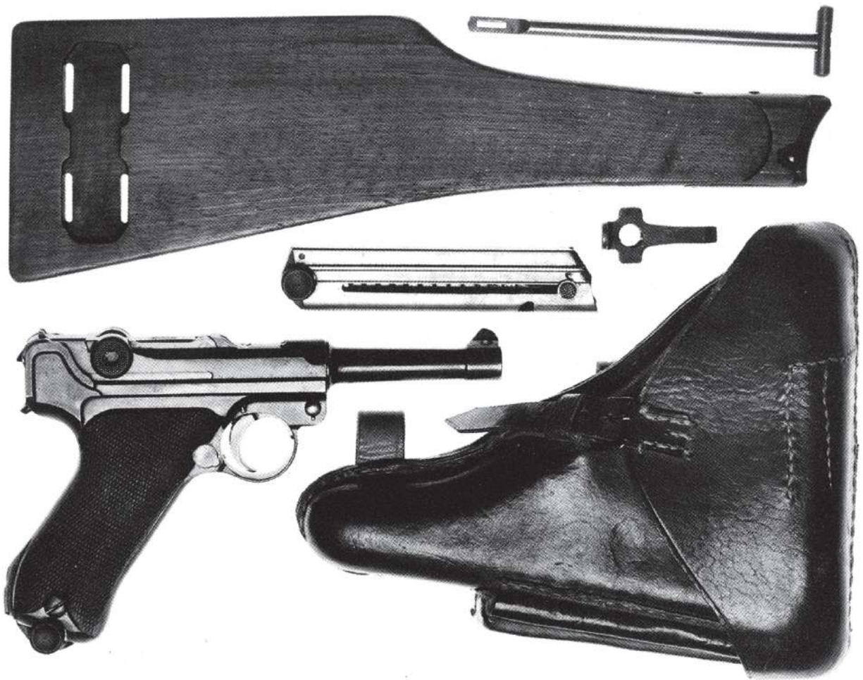
Plate 38 7.65mm m/23 Lugers, made for Finland by Berlin-Karlsruher Industrie-Werke, as DWM was then known, date from the mid 1920s. The holster was attached to the shoulder stock by straps, one of which is visible directly in front of the trigger guard of the pistol. Sotamuseo .
