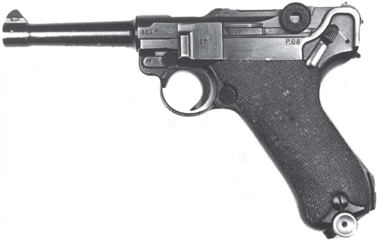
Plate 60 Distinguished by a 'byf' toggle code, this Mauser-made P.08, no.5297h, dates from 1942. Note the identification mark on the left side of the frame ahead of the safety-lever recess. Masami Tokoi.
