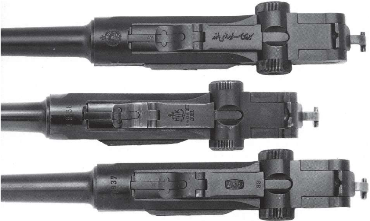
Plates 61–3 The barrel/receiver units of representative Lugers made during the Third Reich. Top to bottom: Mauser-Werke Persian M1 314 no. 1957; Krieghoff no.5220, for the Luftwaffe, 1936; and Mauser-Werke commercial P.08 6488v, 1937. Dr Rolf Gminder.
