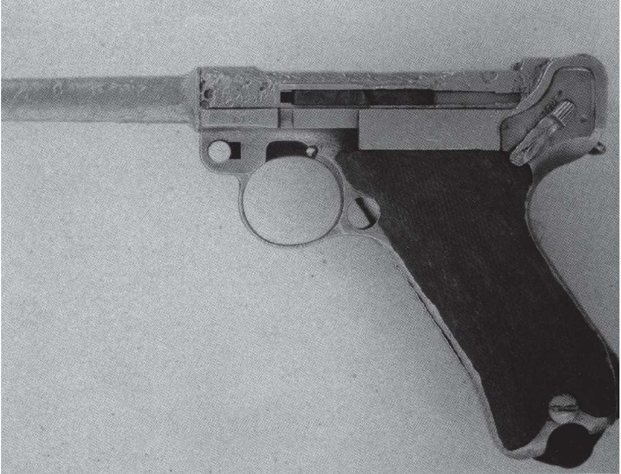
Plates 36, 37 The stern portion of the wreck of U51 (36), being scrapped in Bremerhaven. The four Navy Lugers retrieved from U51 were badly corroded, many of their smallest parts having crumbled away. This particular example (37) is dated '1916' – being virtually brand-new when the submarine was sunk. Ebrbard Schreiber .
