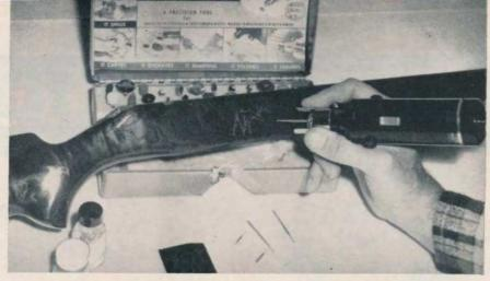
Author uses Dremel Moto-Tool, with fine dental burr, to cut design into the gunstock. Bisonite paste is pressed into cuts and allowed to dry.
