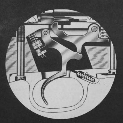
Trigger and sear arrangement on Winchester Model 70
