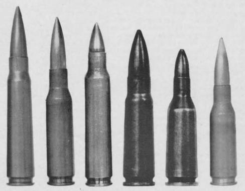
Line-up of some experimental cartridges, left to right: .276 Pederson, 7 mm FN, .224 Winchester, 7.62 mm M-43 Russian, .223 Russian, and the .280-30 British.
