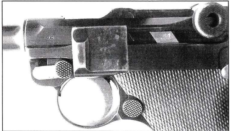
Figure 2. Side view of typical 1916 Commercial Luger. Unusual combination of horizontally-oriented Crown Nitro proof on left side of receiver and 1916 patent safety sear configuration distinguish this model from 1914 Commercial (1908 safety sear configuration) and post-World War I model (vertically-oriented Crown Nitro proof).
