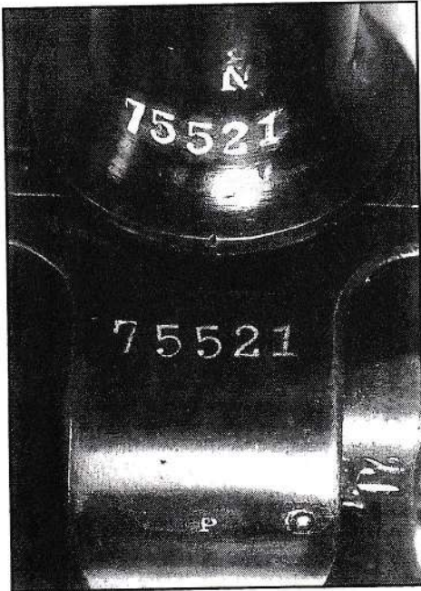
Figure 1. Detail of Typical 1916 Commercial Luger. 1916 Commercial model is identical to 1914 Commercial model, to include horizontally-oriented Crown Nitro proof on left side of receiver and matched, factory-numbered cal. 9 mm proofed barrel, but differs in having 1916-patented sear bar and letter 'P' on underside of frame near take-down lever.
