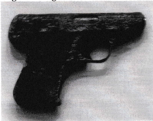
Right side view showing magazine release spring on the right side of the frame.
